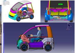
The speed is 20km/h, safe and stable, and the endurance is 80km,
